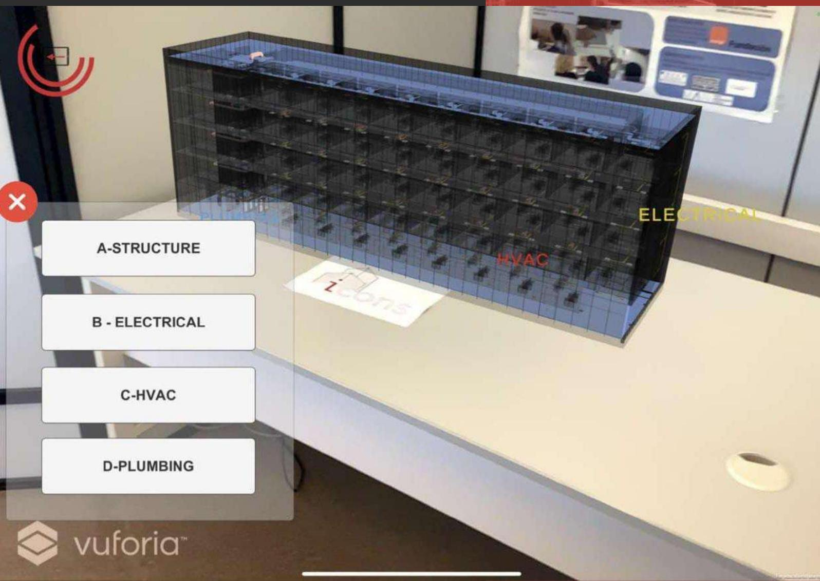
When the system detects this mark it shows a floating virtual mockup of a building. The user can observe the details of the building and the different BIM information just walking around with the mobile device pointing at the mark. If the user move close enough to the mark he can even explore interior details of the building.
