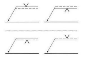
and on the stroke reference line, when welding is done on the side opposite the arrow line Fig. 3
